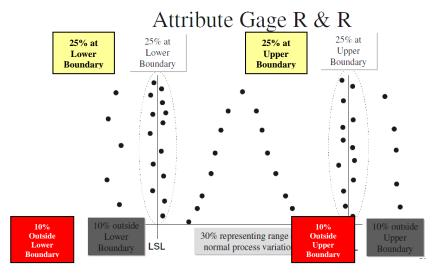
Gages not meeting the acceptance criteria per the AIAG MSA manual shall have an alternate inspection method and a gage improvement plan. This shall be submitted in writing to the Nexteer AQE/SQE for approval.
