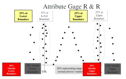
Gage studies should be re-verified at a frequency that is appropriate for gage use and wear. Recommendation – Gage re-verification studies should be completed at the time of calibration
