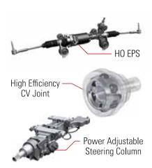
With Nexteer's HO REPS, heavy-duty trucks and light-commercial vehicles can now be converted from hydraulic to electric power steering due to HO REPS' increased steering load capability. HO REPS solves a longstanding consumer pain point for OEMs: where the less-expensive light-duty trucks with EPS offered more safety and comfort features compared to the more expensive heavy-duty trucks that utilised hydraulic steering.
