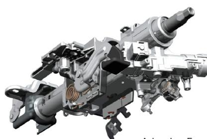
Adaptive Energy Absorption on Manual Adjustable Steering Columns
